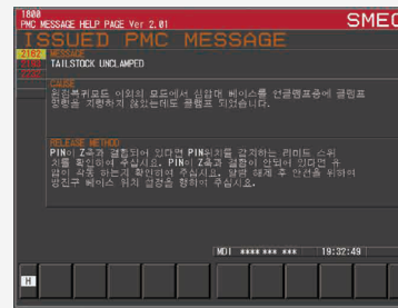
PMC alarm check function
